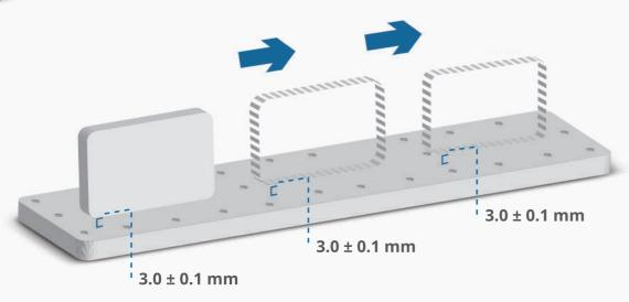
**SoniQi** comes with unmatched FGP technology, which ensures extremely less deviation between jet to bed distance(<**0.1mm**) over the entire printing span and maintains consistent print quality.
